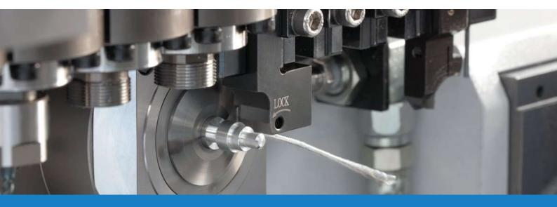
Excellent chip evacuation with y-axis tuning prevents chip entanglement
