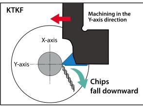
The Y-axis machining direction allows the chips to fall down and away from the workpiece, improving chip evacuation.
