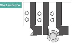
Standard toolholders may be mounted between two Y-axis toolholders.
